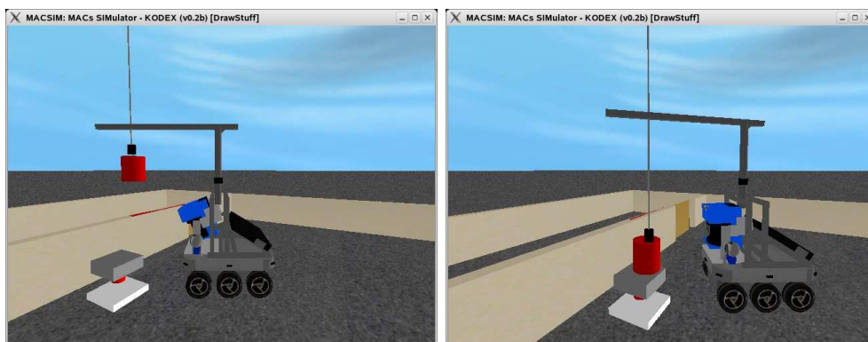
Figure 8: Left: The robot has already lifted the can and has approached the region with the switch. It scans the region to detect the switch-triggerable affordance. Right: The robot has successfully just placed the test object on the switch and the door in the background is opening.
